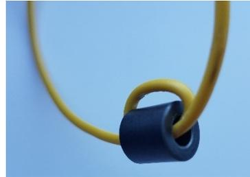
Fig. 1515: Ferrite sleeve and cablet
