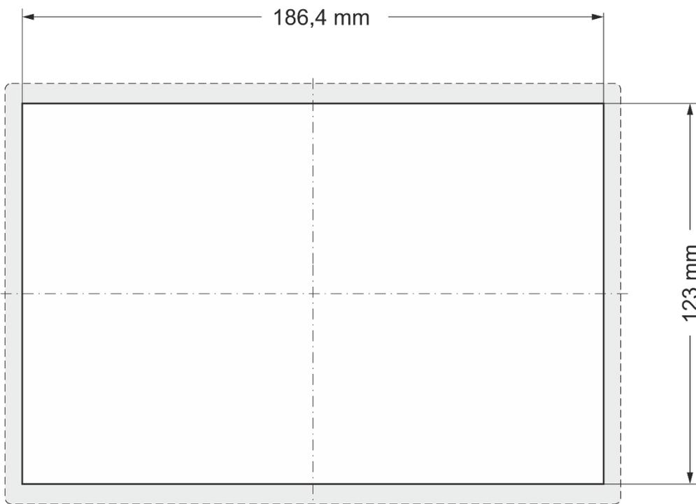
Fig. 33: Installation cut-out DC-Prime 10
